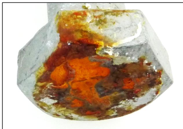
**Figure 5:** test duration: 72 h, detail, sample 5
