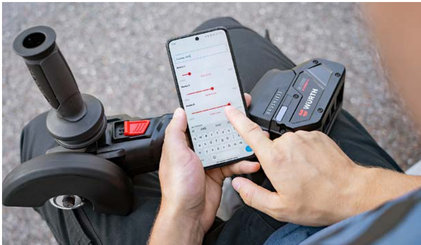
Angle grinder with IoT module for smart and efficient material processing
